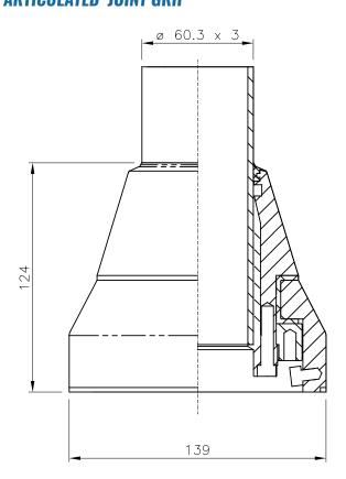
${\rm EN}$  1.4301 (TYPE 304) s/s execution, complete with blue seal to guarantee tightness.
